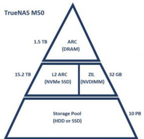
The ZFS Intent Log (ZIL) is where all data to be written is initially stored. These writes are later flushed to disk. The M50 uses NVDIMMs for the ZIL write cache. The NVDIMMs safely provide near-DRAM-speed write caching. This enables the array to quickly acknowledge writes on the front end while efficiently coalescing many random writes into sequential disk operations on the back end.
